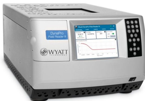
Figure 1: The DynaPro Plate Reader assesses solution quality in standard 96, 384 or 1536 well plates, without perturbing the samples.
