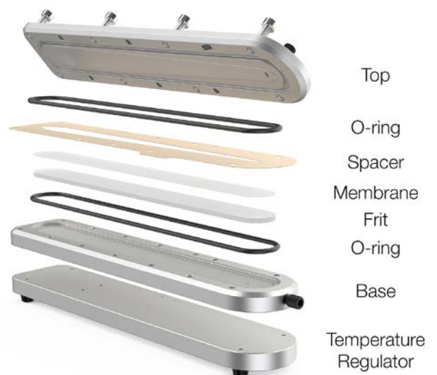
Figure 4. Exploded view of the Eclipse channel. The top and bottom plates are machined from 316 stainless steel for stability. A temperature regulation block added to the bottom plate keeps the temperature stable to improve reproducibility of the retention time.
