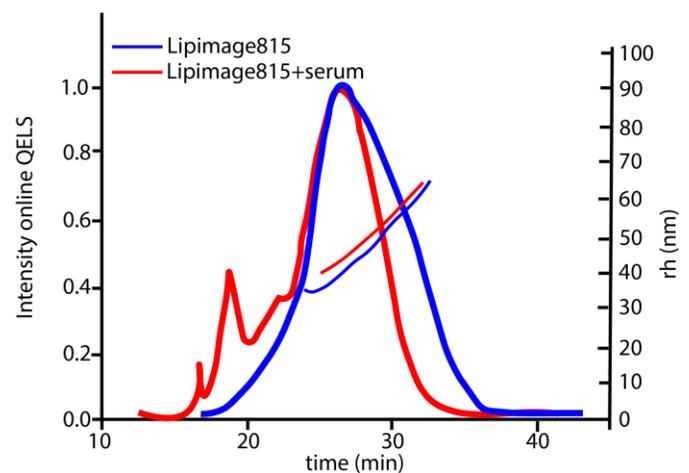
Figure 4. AF4-DLS (QELS) fractogram of lipid nanoparticles incubated with serum. Compared to the original sample, the peak becomes narrower. These slight changes cannot be detected by DLS or NTA. (Figure adapted from Ref. 4)
