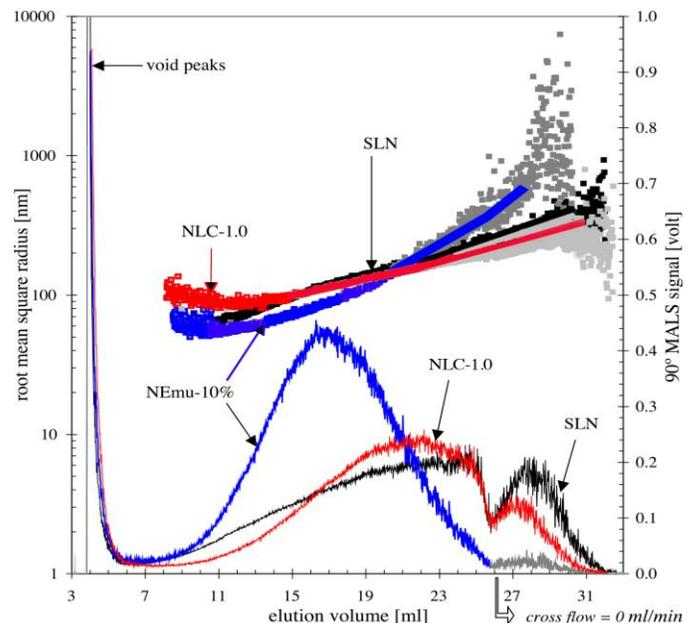
Figure 2. AF4-MALS fractogram of a nano-emulsion (NEMu-10%, blue), SLN (black) and NLC (red) samples. The 90° LS signals are overlaid with calculated RMS radius from MALS. The radius of the nano-emulsion is smaller between 11 and 20 ml elution volume compared to the other two samples, indicating an elongated structure for SLN and NLC (Figure adapted from Ref. 3)
