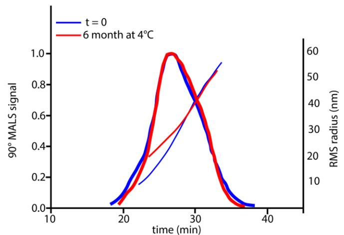
Figure 3. AF4-MALS fractogram of Lipimage815™ which is prepared from a mixture of lipid, lecithin and a dye solution as the active ingredient<sup>3</sup>. The overlay compares the sample at  $t=0$  and after 6 months of storage, indicating an increase of the RMS radius between 23 and 30 minutes of elution time. (Figure adapted from Ref. 4)
