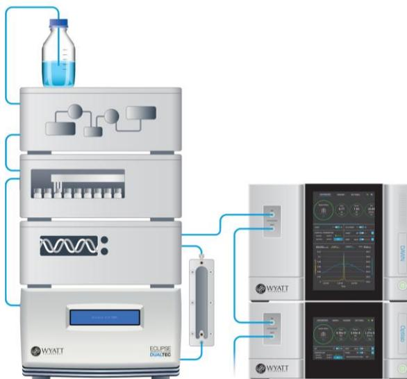
Diagram of an AF4 system comprising HPLC degasser, pump, UV detector and autosampler; Eclipse AF4 control system and separation channel; and MALS and refractive index detectors.
