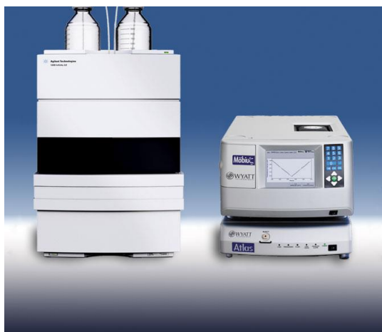
Figure 3. Left: electrophoretic light scattering (ELS) is usually carried out in cuvette-like cells, but when automation of many samples is desired a flow-cell-based instrument with simultaneous ELS and dynamic light scattering capability may be connected to an autosampler. Bottom: graph shows drift vs time under a field of alternating polarity, and the fitted mobility result.
