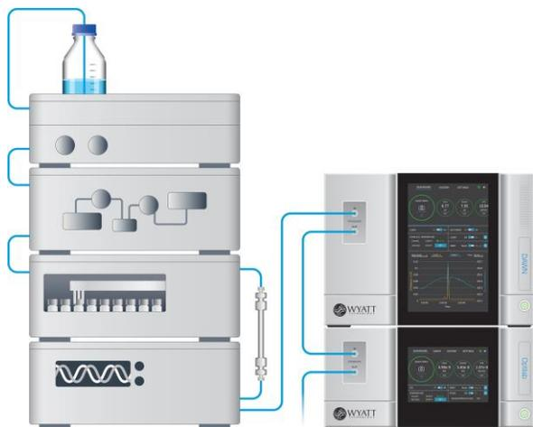
A complete SEC-MALS system comprises the HPLC including the UV detector, SEC column(s), MALS and RI detectors. Control, data acquisition and analysis are performed by ASTRA.
