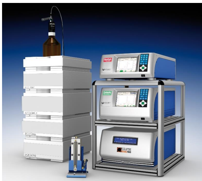
The Wyatt Technology Eclipse™ DualTec FFF system can be coupled with a DAWN® HELEOS® II MALS and Optilab® RI detectors to characterize particle size and aggregation.
