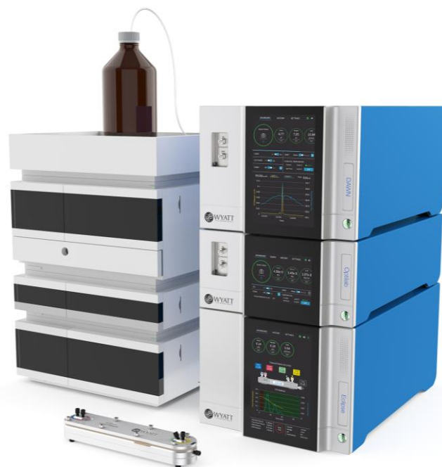
Figure 2. An FFF-MALS system comprises HPLC components together with an Eclipse FFF flow controller and separation channel, a DAWN MALS instrument and Optilab differential refractometer, plus VISION and ASTRA software for control, data acquisition and analysis.
