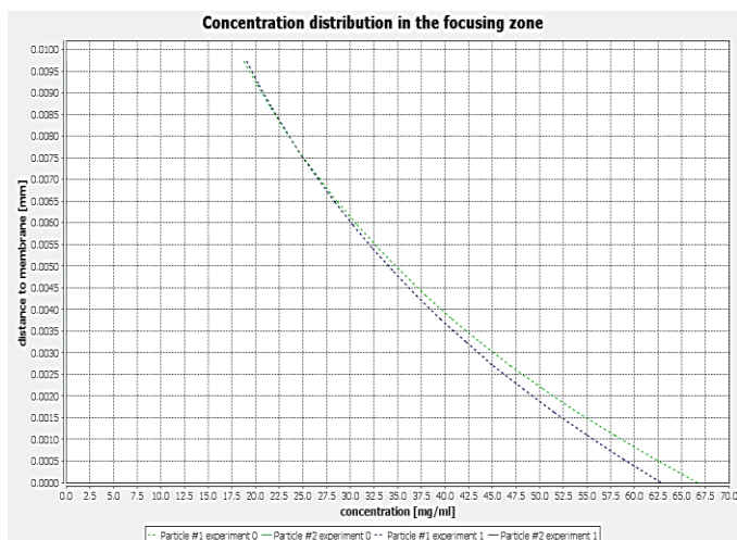
Figure 2. ISIS model of concentration distribution in the focusing zone. The plot shows the concentrations achieved at the membrane during the separation.
