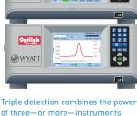
Triple detection combines the power of three—or more—instruments to determine absolute molecular weights, sizes and viscosities.
